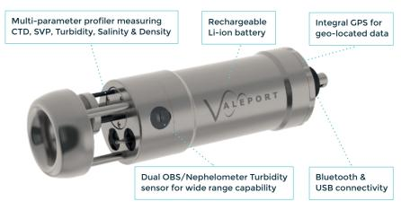
Valeport's Turbidity technology is essentially two sensors in one. The first is a "classic" nephelometer, using a 90° beam angle for turbidity levels between 0 and 2,000 NTU. The second sensor uses Optical Backscatter (OBS) for turbidity levels up to 10,000 NTU. The sensors output data separately and simultaneously at a programmable rate. This means that there is no need to switch ranges as conditions vary. Intelligent sampling and the use of a 24 bit ADC eliminates the need to switch gain.
