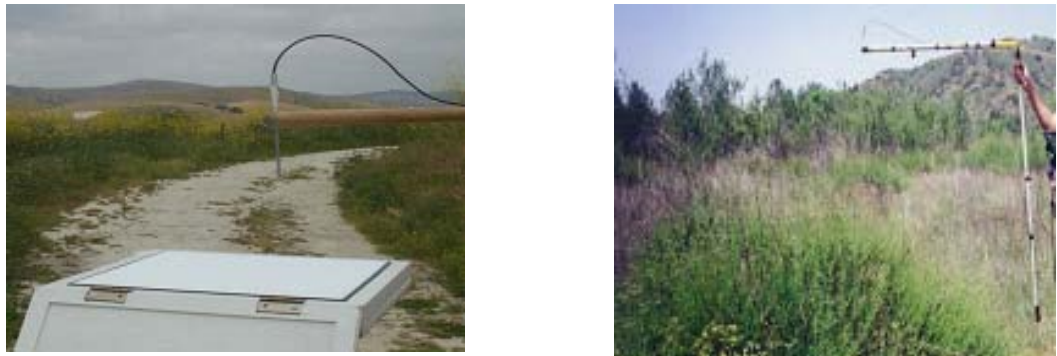
Figure 3. Using UniSpec-SC in the field to measure ecosystem optical properties. Reference measurement (left) and target measurement (right) are required in order to calculate the reflectance. (Photo courtesy of Dr. John A. Gamon at California State University, Los Angeles)
