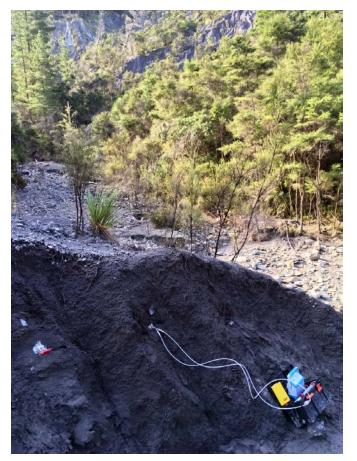
**Figure 2.** An example of the new method (EGM-5 Portable CO<sub>2</sub> Gas Analyzer connected to a chamber drilled in the rock face [2], through the MS<sup>3</sup> monitoring-sampling system [3]) being used in the Waiapu River catchment, New Zealand. (© *R. Hilton*)
