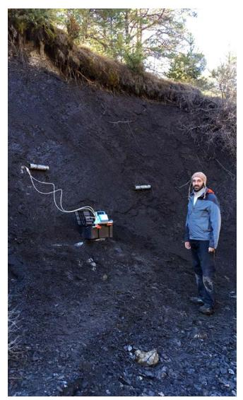
**Figure 1A.** EGM-5 Portable CO<sub>2</sub> Gas Analyzer connected to a chamber drilled in the rock face [2], through the MS<sup>3</sup> monitoring-sampling system [3], while we measure CO<sub>2</sub> efflux from sedimentary rock in the Laval stream catchment, Draix, France. (© *R. Hilton*)
